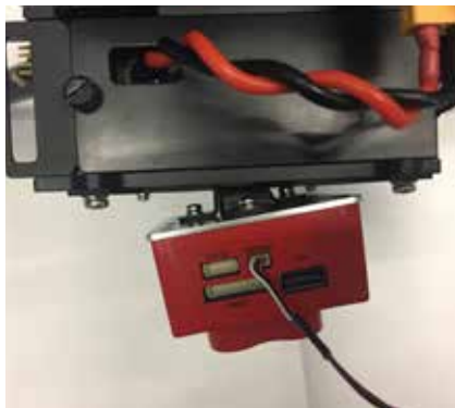
RedEdge-M connector of BEC plugged into RedEdge-M power port
