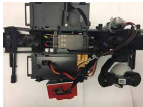
BEC attached to airframe using included VHB tape and zip ties.
